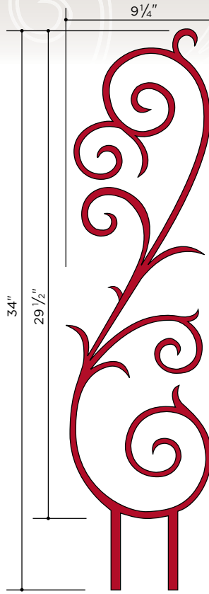
● 538* Malleable Iron 7.0 lbs Cross Section: Scroll – 5/8" x 7/16" Ends – 1/2" x 1/2"
