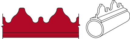
● 4445 Steel .688 lb/ft Loafer rail fits over pipe or flat surface to discourage lounging or skating on fences, planters, railings, or storefronts.
